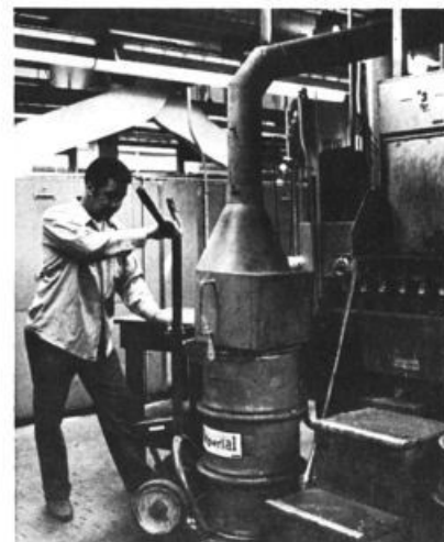
Marion Campfield removes a drum of lead dross near the Supermatic machine lead pot in Stereotyping.
