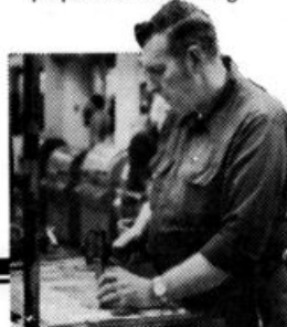
With a block and hammer, stereotyper BILL VARNEY works the chase in preparation for matting.
