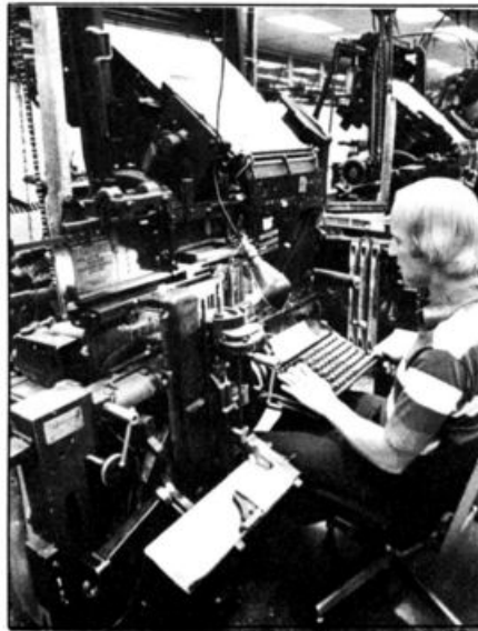
The linotype machines produce slugs of type for the hot type printing process; in the 1980s the entire paper will produced by cold type.
