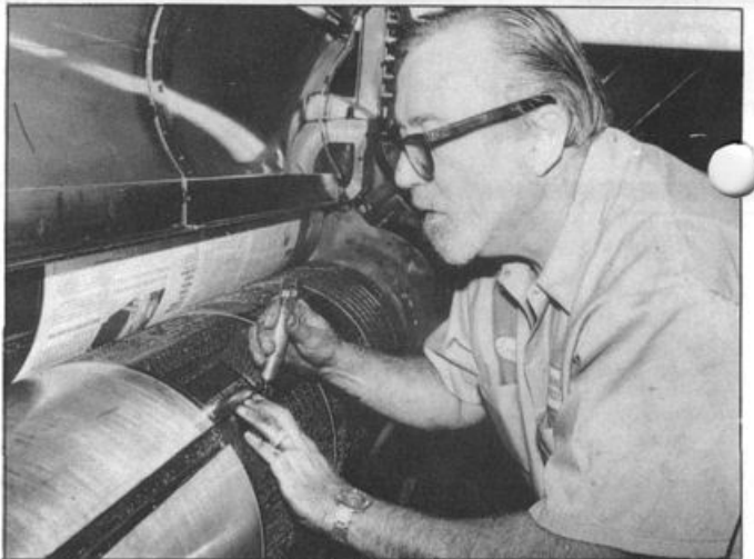
Southeast Plant Press room foreman JIM LOGAN locks the final plate on press before starting the presses.
