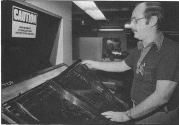
In the plant's Engraving Department, engraver MARTIN OBERMAN readies a negative for exposure by placing it on a sheet of glass. The glass is then placed over the plate, and liquid polymer is poured between the two.
